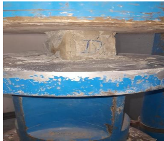
Fig 10: Compressive strength test of Geopolymer Mortar Cubes.
